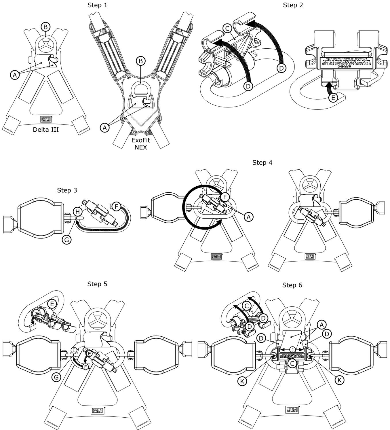
**A** - Web Straps **B** - Dorsal D-Ring **C** - Connector Insert **D** - Clamps, Connector Insert **E** - Gate, Connector **F** - Nose, Connector
