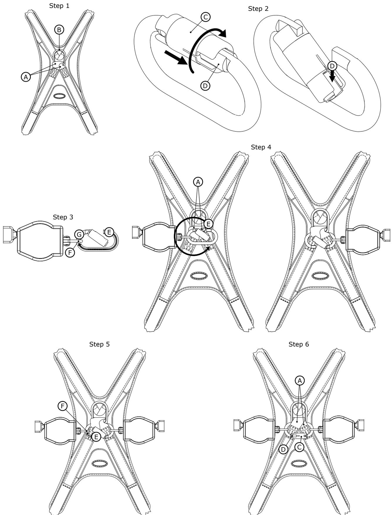
**A - Web Straps B - Dorsal D-Ring C - Locking Sleeve, Connector D - Gate, Connector E - Nose, Connector F - Swivel Eye, SRL**
