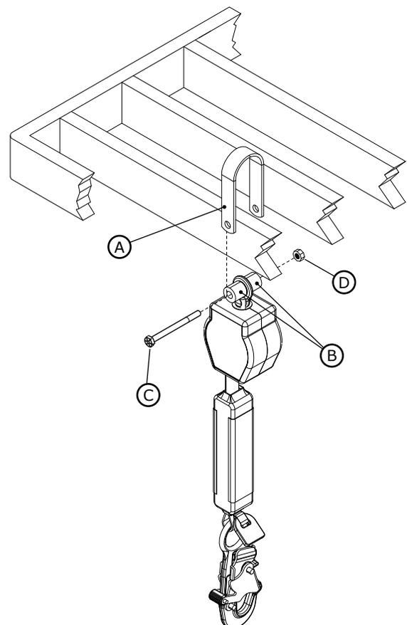
A - Anchorage B - Connector C - Tie-Off Adapter
