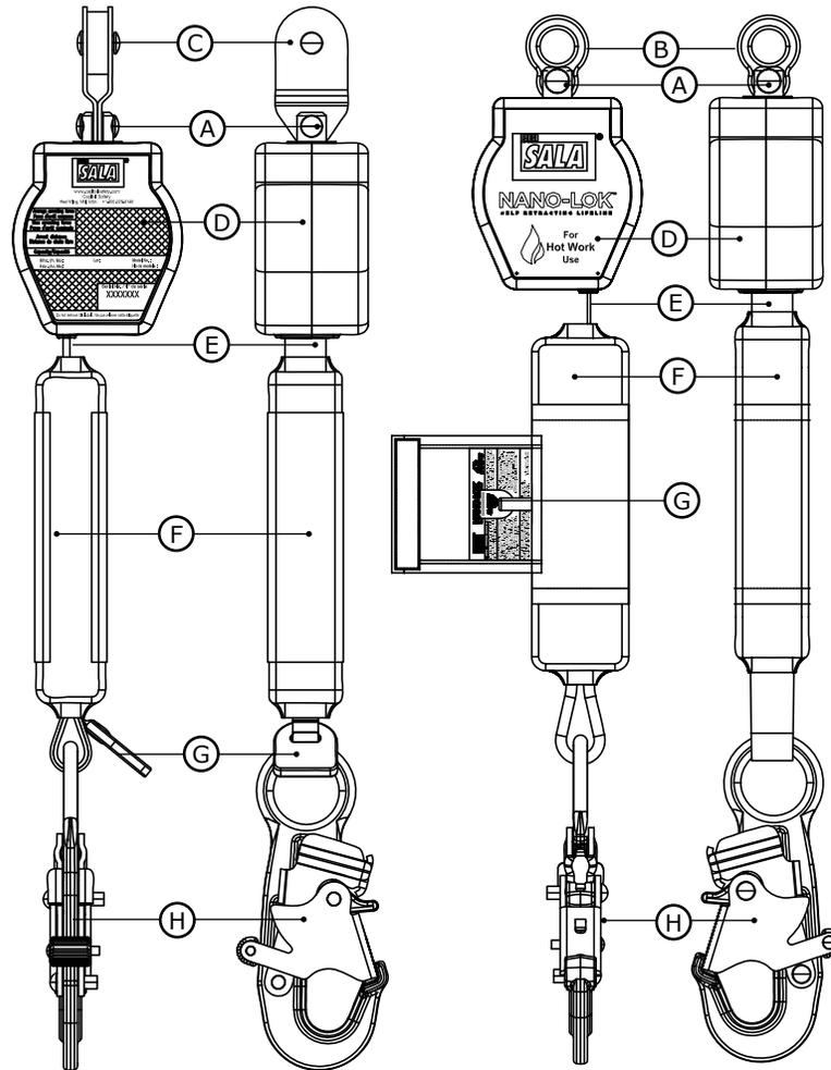
**A** - Swivel **B** - Swivel Eye **C** - Integral Connector **D** - Housing **E** - Web Lifeline **F** - Load Indicator **G** - iSafe™ RFID Tag
